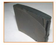
The main characteristics of pyrolithic graphite are: chemically inert, high purity (99.999 %); durable up to 500 °C in air, up to 2500 °C in 0.1 torr vacuum, up to 3500 °C in atmosphere (Ar, He, N); impermeable; non-dusting; resistant to thermal shock; easily machined.
